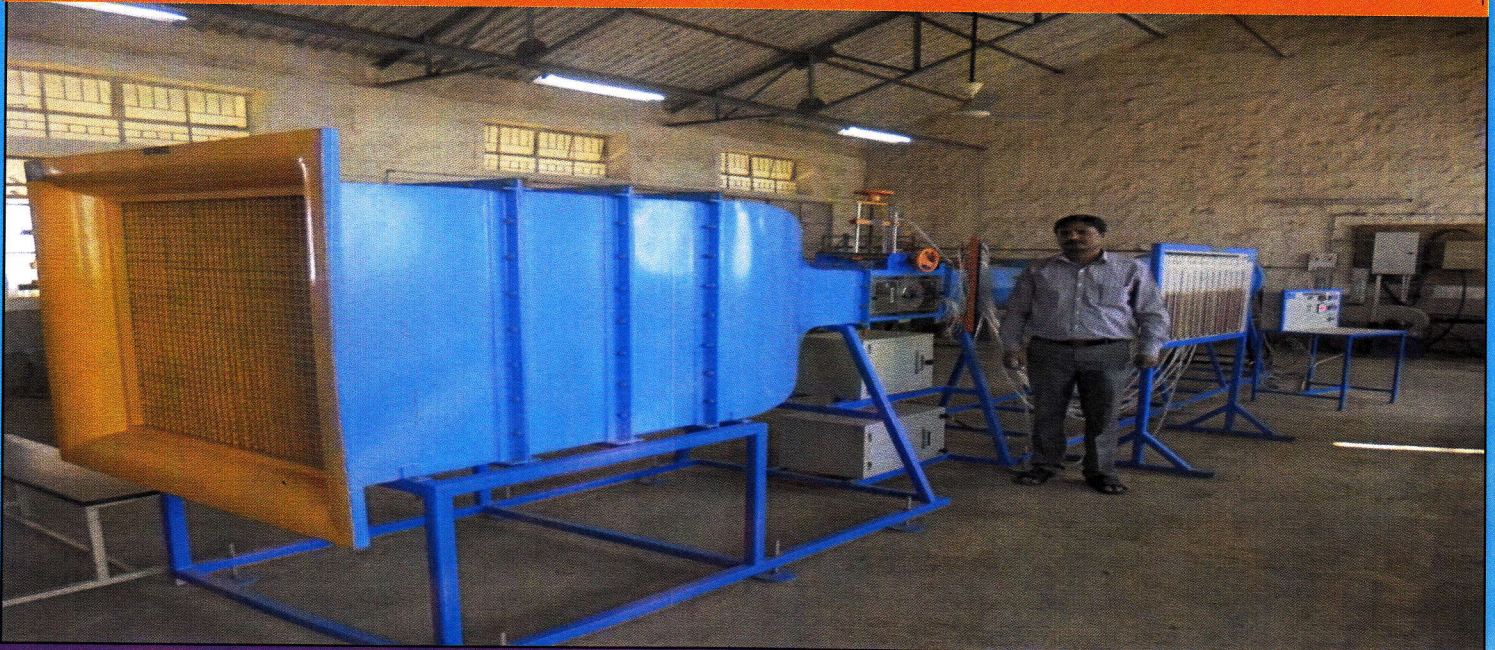
The VGST, Government of Karnataka catalyzed Wind Tunnel of Test Area (300 X 300 X 1000) mm Successfully Installed in the Department to Promote Research on Aerodynamic by The Programme Coordinator Dr. S.N. Topannavar.
